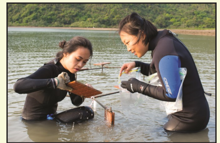
Deploying settlement plates as part of a monitoring program in Yueng Shui O, Hong Kong. Credit: Lori Cheung
